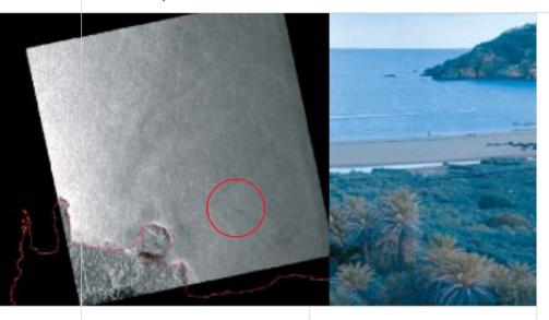
To fight oil pollution, the PROMED project is based on the development of the synthetic aperture radar imaging and very high resolution radiometry. Circle on left picture indicates the location of a possible oil slick.
